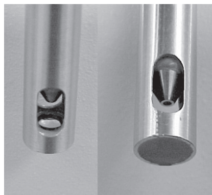
Figure 2. View of concave mirror (left) and fiber optic source in probe tip (right).
